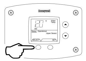
Step 2: For water heaters using two temperature sensors, pressing the "Select" button again displays the Upper Sensor temperature reading. "Upper Sensor" will be displayed in the lower right side of the status window of the water heater display.
